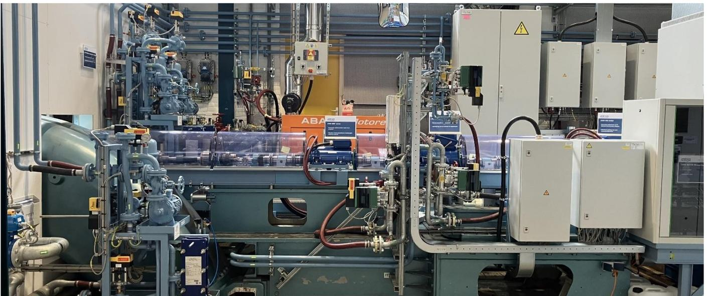
The physical Zero Emission Lab, having a mechanical electric propulsion drive, containing sophisticated electrical power distribution powered by a PEM fuel cell, a modern dual fuel generator set and super capacitors.
